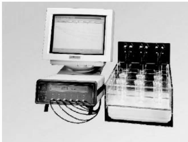
Figure 3 The Strathkelvin Activated Sludge Respirometer which utilises 6 oxygen electrodes connected via an interface to the pc loaded with dedicated respirometry software.
