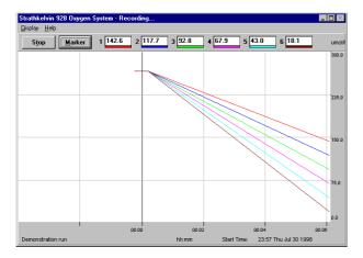
As the experiment progresses, oxygen concentration is plotted against time and is viewed scrolling across the screen. Annotated event markers can be incorporated to highlight any experimental manipulations during the recording.
