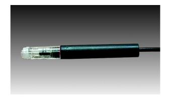
The Clark type electrode consists of a platinum cathode and silver/silver chloride anode connected by a buffered potassium chloride electrolyte solution.
