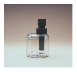
The RC300 and RC350 cells consist of a glass water jacket housing the sample chamber and electrode parking tube.
