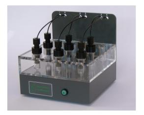
When operated with the 929 Oxygen meter this complete 6 cell respirometry system enables replicate measurement of dissolved oxygen and respiration rates.
